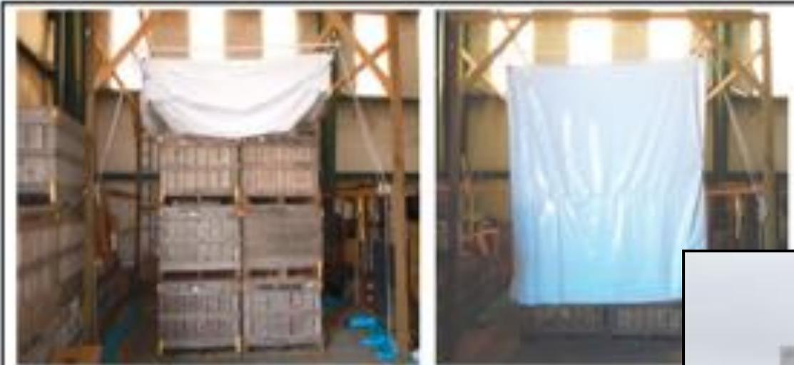
Figure 4. The Adjustable Apple Test (<http://theblaworks.com/>) has a four by six footprint and can hold a bin of fruit at a time. The tent is raised or lowered to minimize dead space and maintain the active ingredient at an effective level for the duration of the 24-hour treatment period. It is easily set up on a pallet base with a water bladder.
